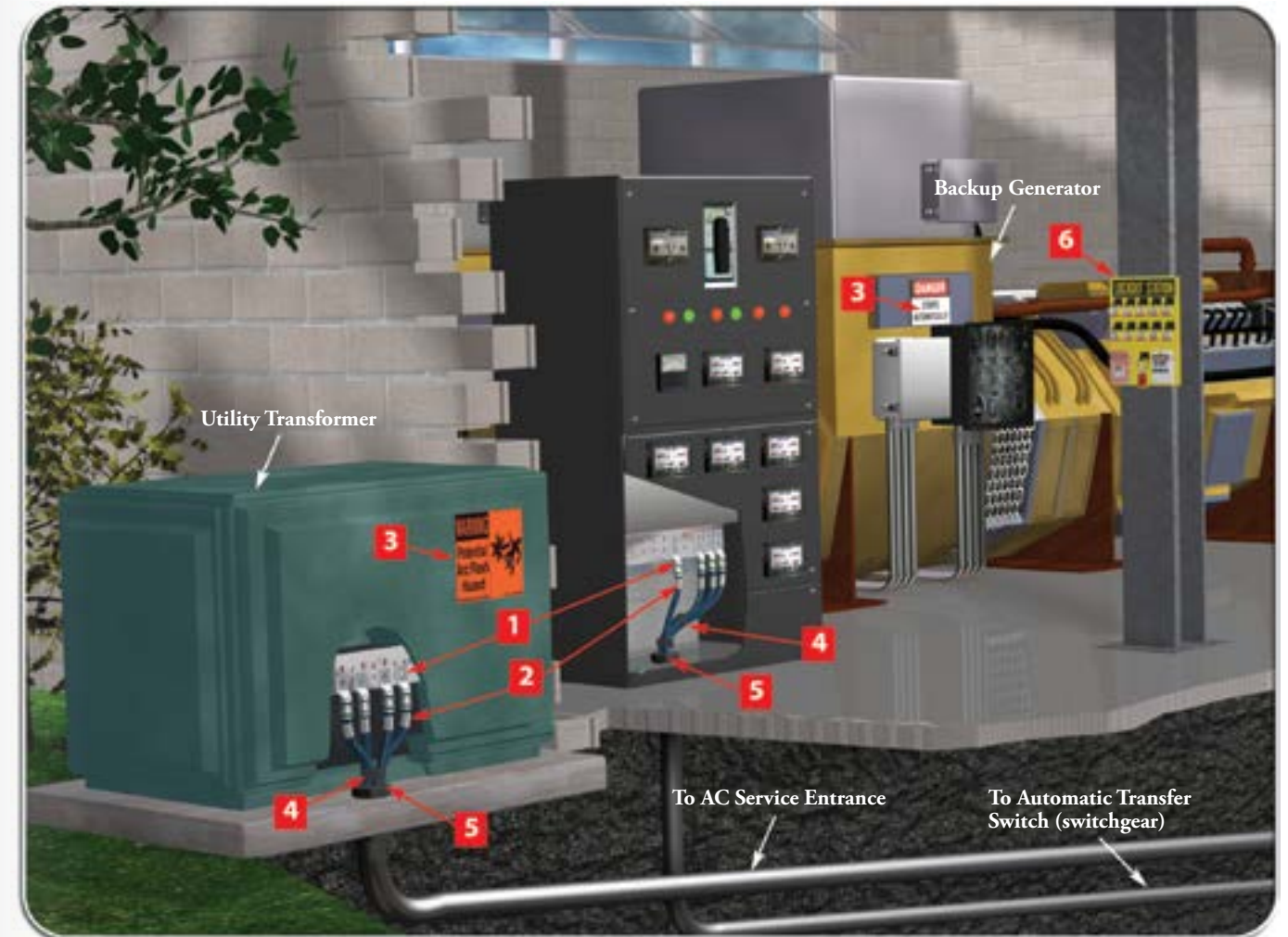
The utility transformer provides the main power to the system. In the event of an interruption, the backup generator provides power.
